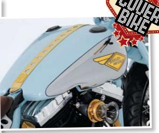
THE BRASS TANK-**RETAINING STRIP BOTH KEEPS THE TANK DOWN** AND, AGAIN, ADDS TO THE VINTAGE FEEL OF THE WHOLE PROJECT
