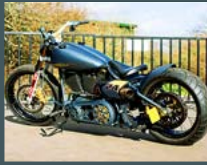
CYCLE The front end is influenced by a mountain bike, with its RockShox-style white forks
