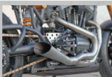
2-1 header pipe with a Vance and Hines exhaust can is fitted
