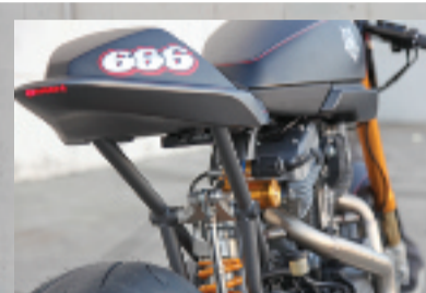
Simple tubular support with hand-beaten aluminium tail unit
