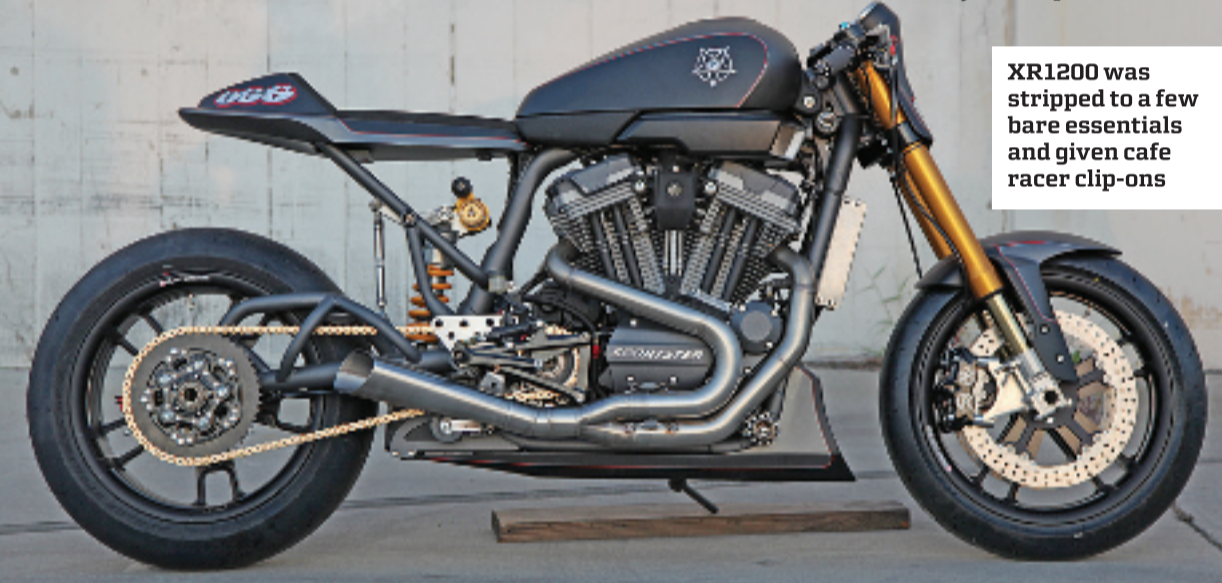
Simple tubular support with hand-beaten aluminium tail unit
