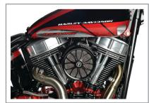
The SS&C-built 120 cubic inch Screamin Eagle motor sports lots of performance goodies, including high-volume fuel injectors, anodized pushrod tubes and Covington rocker covers. The SS&C Red Edition engine case is joined by a cam cover coming from Roland Sands Design's Clarity line.
