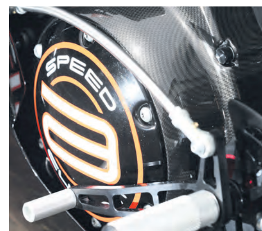
Spirits rearsets and a modified Harley XR1200R engine
